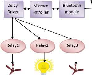
Fig: 2. Block diagram of Receiver section
